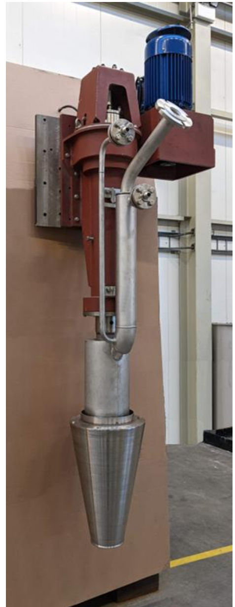
Figure 11: Stamicarbon vibro-prilling bucket
